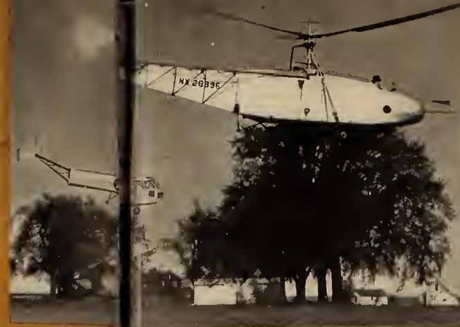
The conventional model of the helicopter, piloted by its developer, flies low over a Connecticut meadow with the Army's new model in the background. Note that the Army version has an enclosed cockpit and fully-covered fuselage.
